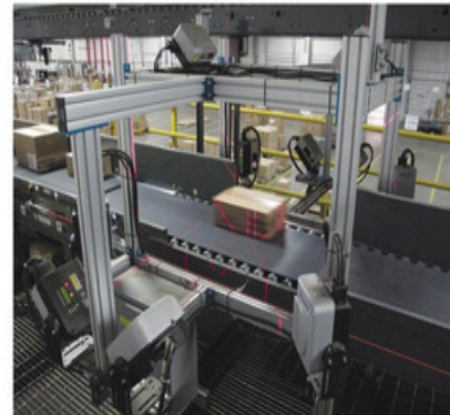
Driven by sophisticated automation software and controls, multiple integrated distribution and fulfillment systems (including laser-based identification and dimensioning technologies) communicate in a warehouse to identify and route items and parcels through the facility and out to a customer.
