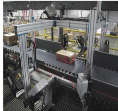
Driven by sophisticated automation software and controls, multiple integrated distribution and fulfillment systems (including laser-based identification and dimensioning technologies) communicate in a warehouse to identify and route items and parcels through the facility and out to a customer.
