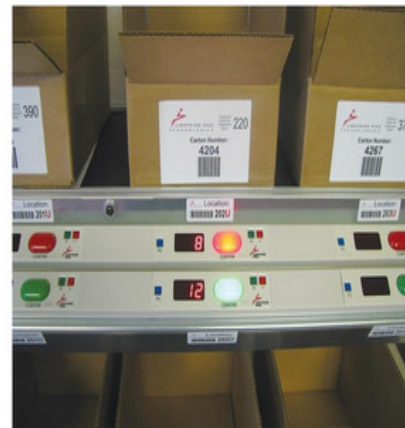
Pick-to-Light systems use light indicators for sorting and control of merchandise.
