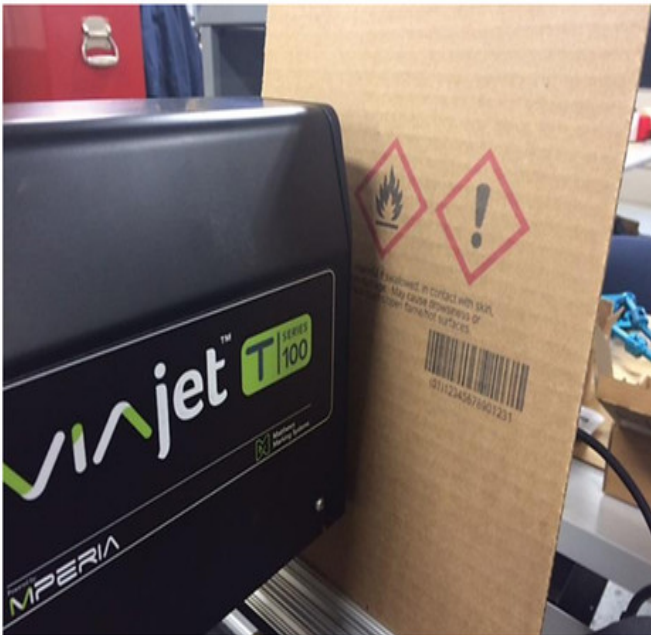
Non-contact ink-jet printing units apply print on products.
