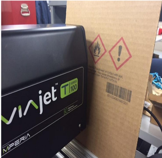
Non-contact ink-jet printing units apply print on products.
