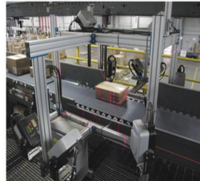
Multiple integrated distribution and fulfillment systems (including laser-based identification and dimensioning technologies) communicate in a warehouse to identify and route items and parcels through the facility and out to a customer.
