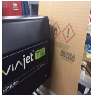
Non-contact ink-jet printing units apply print on products.
