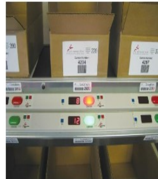
Pick-to-Light Systems utilizing light indicators for sorting and control of merchandise.
