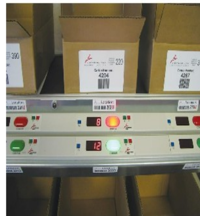
Pick-to-Light Systems utilizing light indicators for sorting and control of merchandise.
