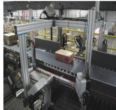
Multiple integrated distribution and fulfillment systems (including laser-based identification and dimensioning technologies) communicate in a warehouse to identify and route items and parcels through the facility and out to a customer.
