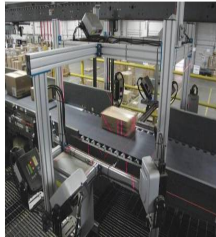
Multiple integrated distribution and fulfillment systems (including laser-based identification and dimensioning technologies) communicate in a warehouse to identify and route items and parcels through the facility and out to a customer.
