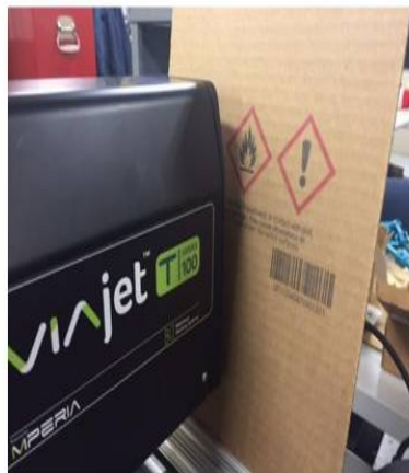
Non-contact ink-jet printing units apply print on products.
