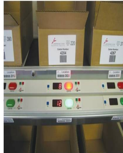
Pick-to-Light Systems utilizing light indicators for sorting and control of merchandise.
