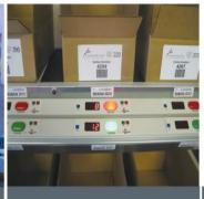
Industrial's **Pick-to-Light Systems** utilizing light indicators for sorting and control of merchandise.
